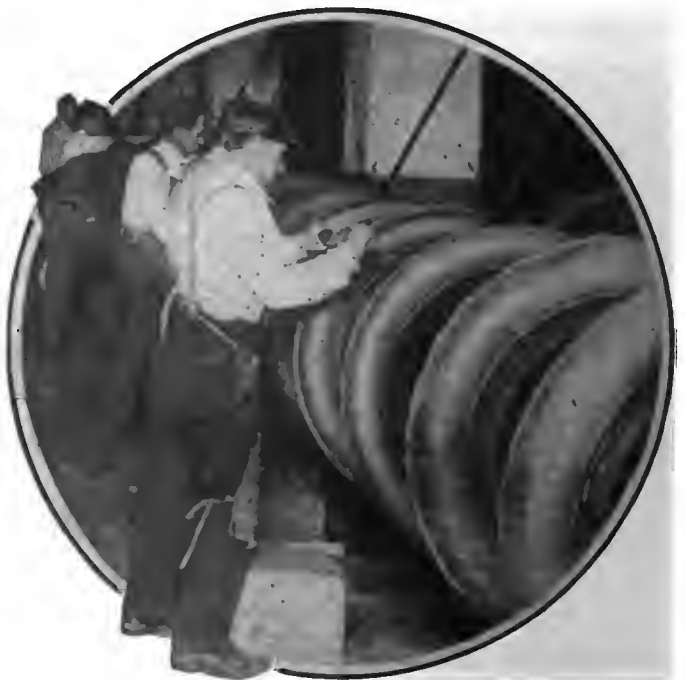
Each tire is buffed before the tread is put on
